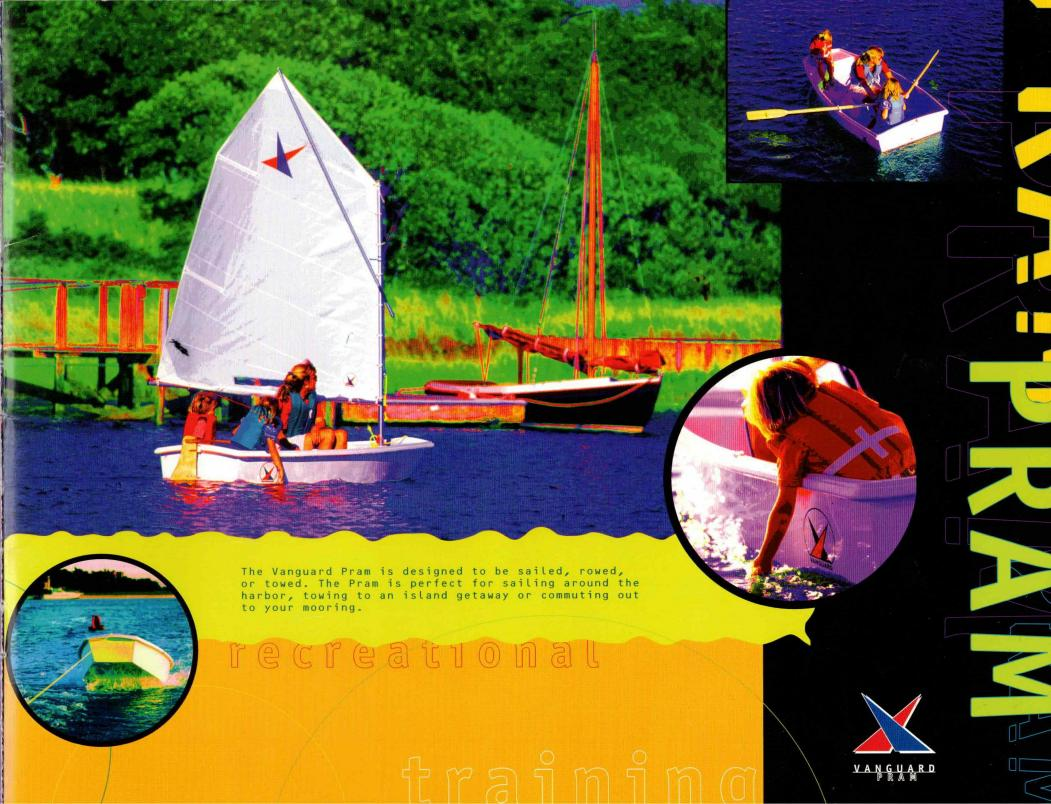
In rowing mode, the Pram has built-in seating in the form of three fiberglass seats that double as buoyancy tenks. In sailing mode, the Pram features a molded-in mast step and a simple rig and blade package. The stable hull shape and bulletproof, unsinkable construction make the Pram a fantastic thoice for new sailors.
